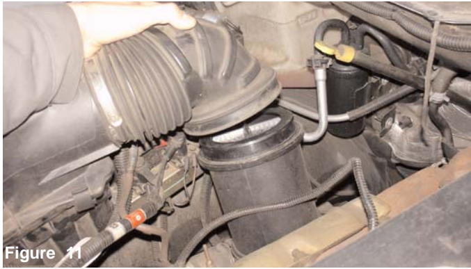
Figure 12 Pull the entire air box and flexible air intake duct from the engine compartment.
