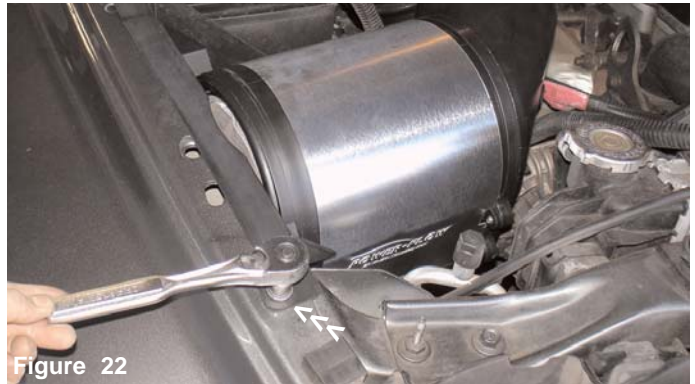
Figure 20 The air box and bracket is now lowered into the engine compartment. Align the bracket holes with the tapped holes on the fender well.
