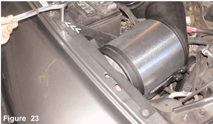
Figure 21 The air box is carefully lowered into the engine compartment with the bracket is placed over the fender well as shown above.
