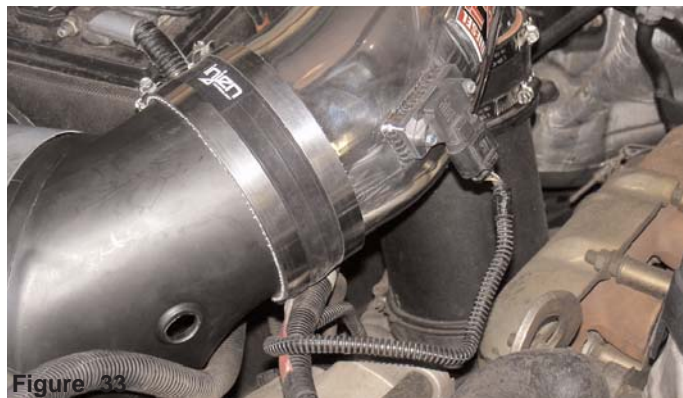
The electrical sensor clip is now firmly secured to the mass air flow sensor.
