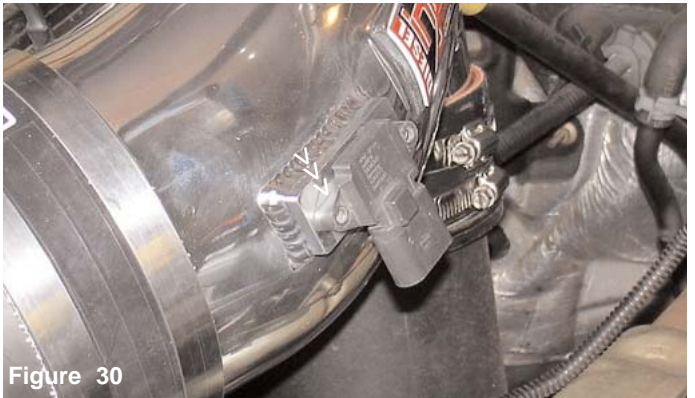
The MAFS is carefully pressed into the sensor adapter.
