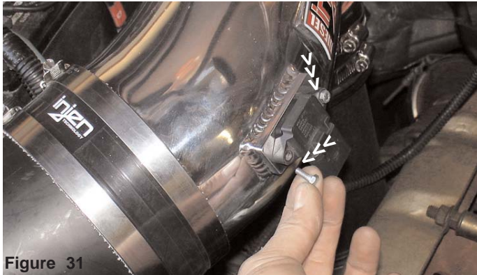
Use the m4 x 16mm button head screws to fasten the mass air flow sensor to the sensor adapter.
