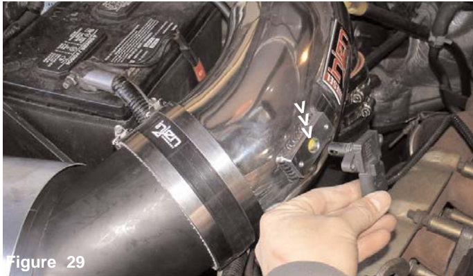
Insert the mass air flow sensor into the machined adapter. Prior to positioning the MAFS, rub a small amount of light oil on the O-ring to prevent the O-ring from kinking or ripping.
