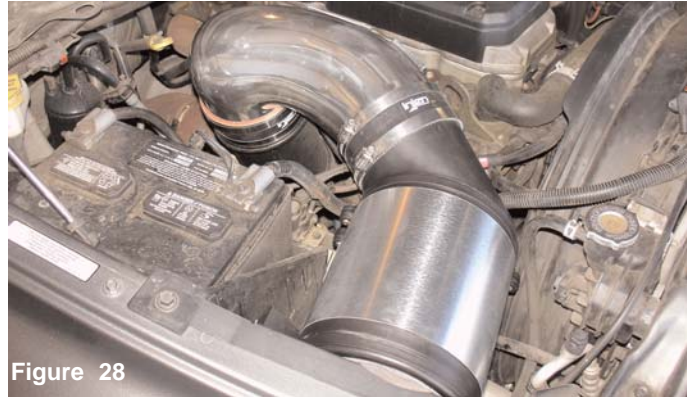
Align the entire cast intake and air box for best possible fit.
