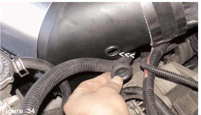
Press the new air restrictor gauge into the pre-drilled 3/4" hole on the plenum. Rotate the grommet so that the grommet is free from any lines.
