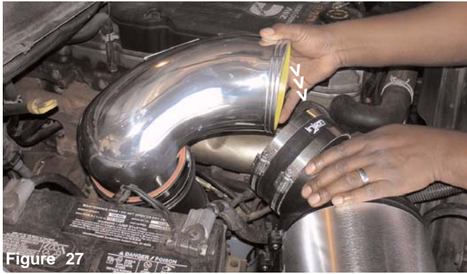
Once the intake has been align, continue to insert the intake into the plenum hose.
