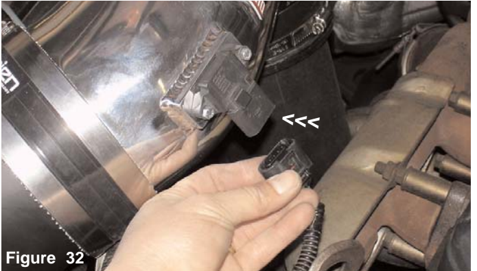
Press the electrical sensor clip over the MAFS until you hear them snap together.
