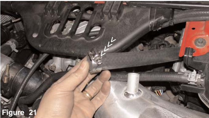
Figure 22 The clamp is now fastened over the 19mm hose as shown above.
