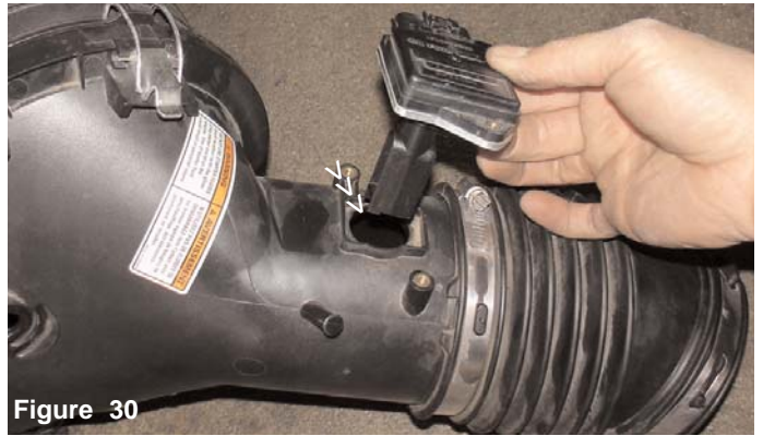
Figure 30 Once you have removed the bolts, continue to pull the mass air flow sensor out of the sensor housing.
