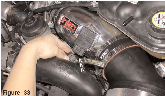
Figure 33 Reconnect the electrical sensor clip to the mass air flow sensor. Press the harness clip over the mass air flow sensor until you hear them snap together.
