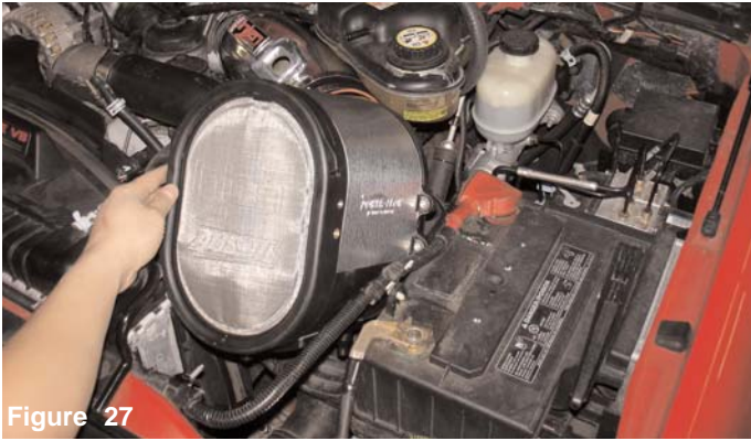
Figure 27 The plenum outlet is pushed into the 5 1/2" straight hose and the pegs on the mounting plate are aligned to the stock grommets. Gently push down on the air box until its sitting flush.
