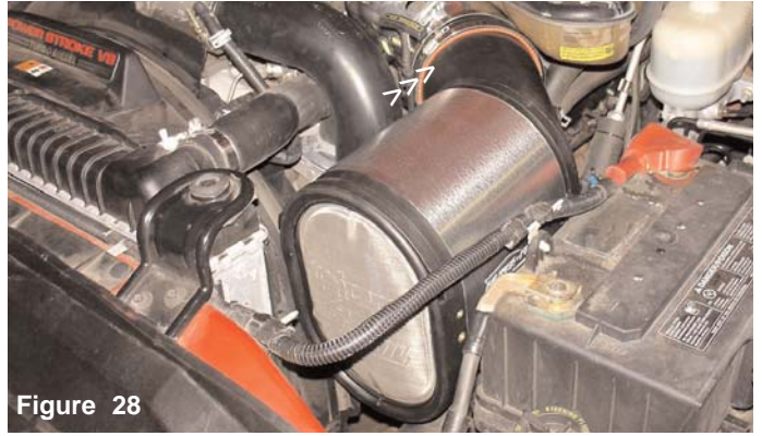
Figure 28 The Injen/AMSOIL air box should now be sitting flush over the stock grommets and the plenum should be pressed into the 5 1/2" straight hose.
