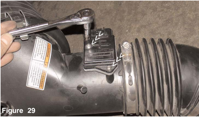
Figure 29 Use the T20 torx bit in this kit to loosen and remove the bolts on the mass air flow sensor.
