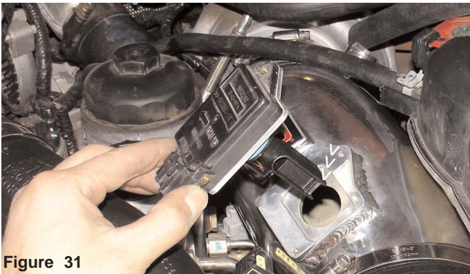
Figure 31 The mass air flow sensor is pressed into the machined sensor housing located on the cast intake. Rub a small amount of light oil around the O-ring to prevent the O-ring from kinking up in the sensor opening.
