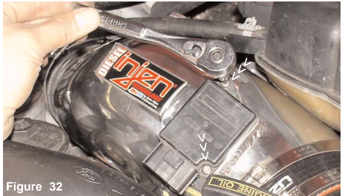
Figure 32 Use the stock bolts to fasten the mass air flow sensor over the machined sensor adapter.
