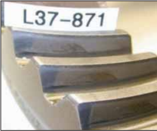
Ring gear exhibits very low wear.
